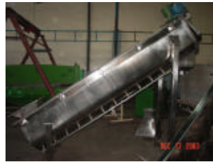
INCLINED SCREW W/ STEAM INJECTION
